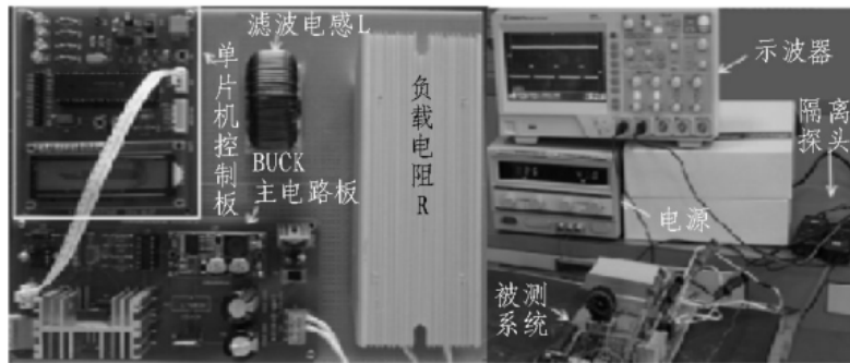
Figure 9 Experimental hardware and test system diagram
